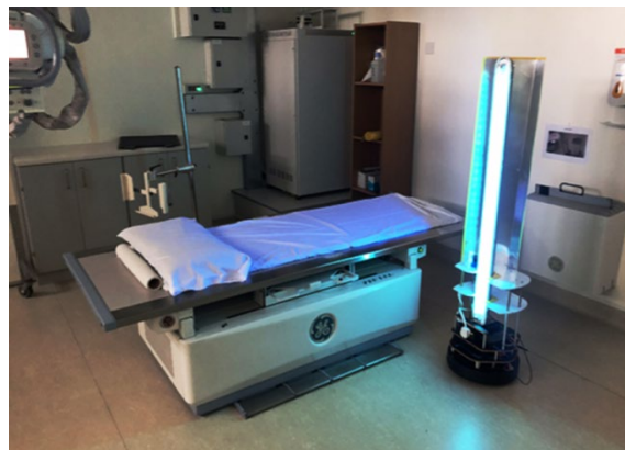
Figure 62. Violet is a robot designed to help in sanitation of hospital rooms and can be used in closed spaces like stores and in offices. Using UV light, it can kill the coronavirus and has a smart detection system to switch off the UV light if a human shows up. Image credit: Akara Robotics
