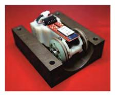
Figure 9: Assembled robot in a 50mm I.D. half-pipe.
