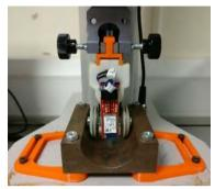
Figure 10: Single column linear force tester with a 10N load cell.
