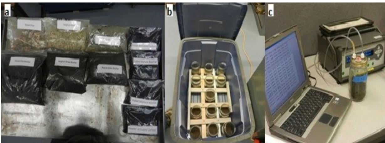
Figure 4-1 Photographs of the experiment: (a) amendment materials, (b) glass containers with the compacted moist manure, within a plastic container with water at the bottom to maintain constant manure water content, and (c) measurement set up.
