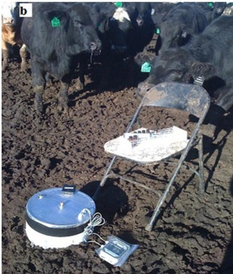
Figure A-3 Static flux chamber in the field: (a) set up and (b) gas sampling.
