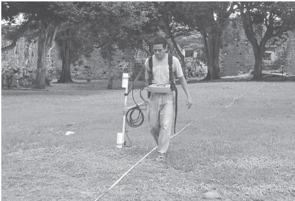
Fig. 2: Caesium magnetometer system (G-858 of Geometrics) in gradiometer mode.
