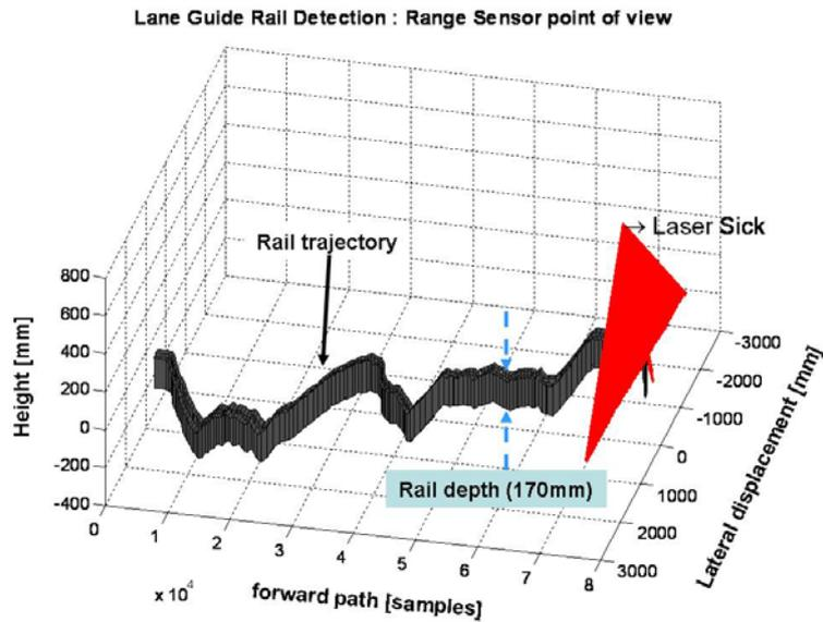
Figure 6. Test lane detection using laser sensor (SICK).
