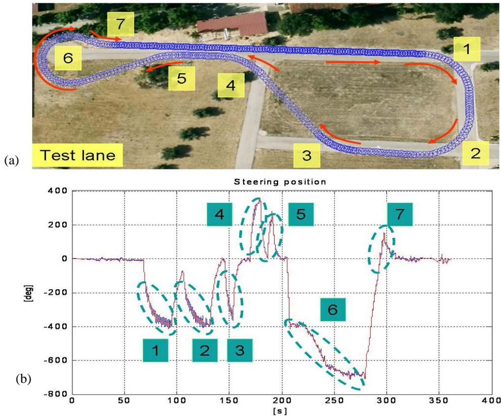
**Figure 5.** (a) New test lane over the old road at the IAI-CSIC; (b) Steering wheel position during a experiment conducted on the new test lane.
