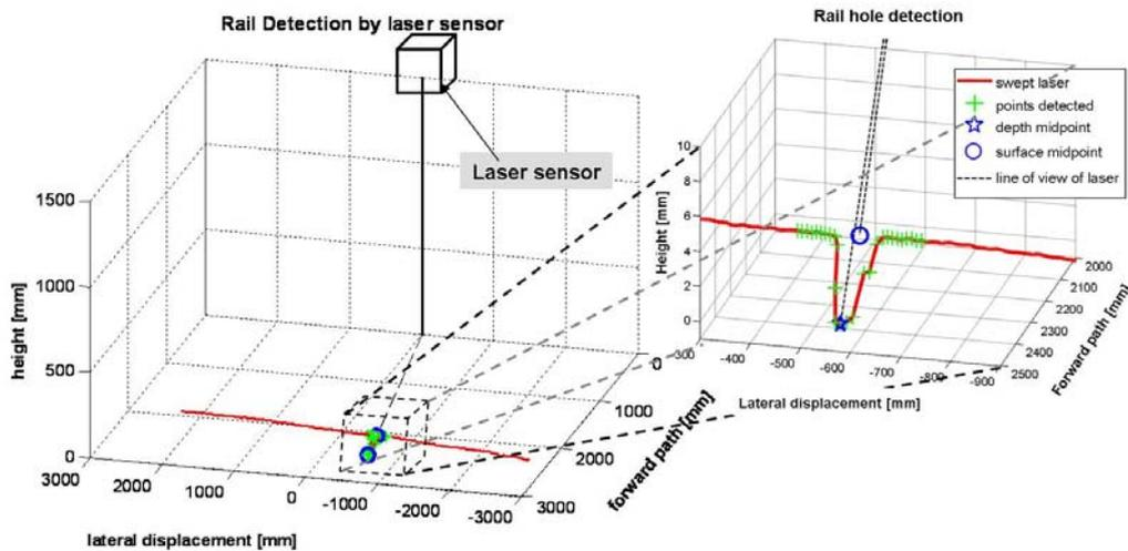
Figure 7. Detection of rail depth by means of laser sensor.
