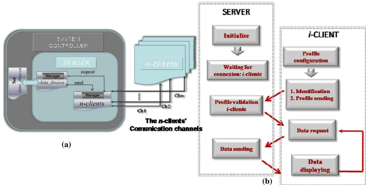
**Figure 2.** (a) General diagram of the remote system communication; (b) Block diagram of communication sequence between server & *i-client*.
