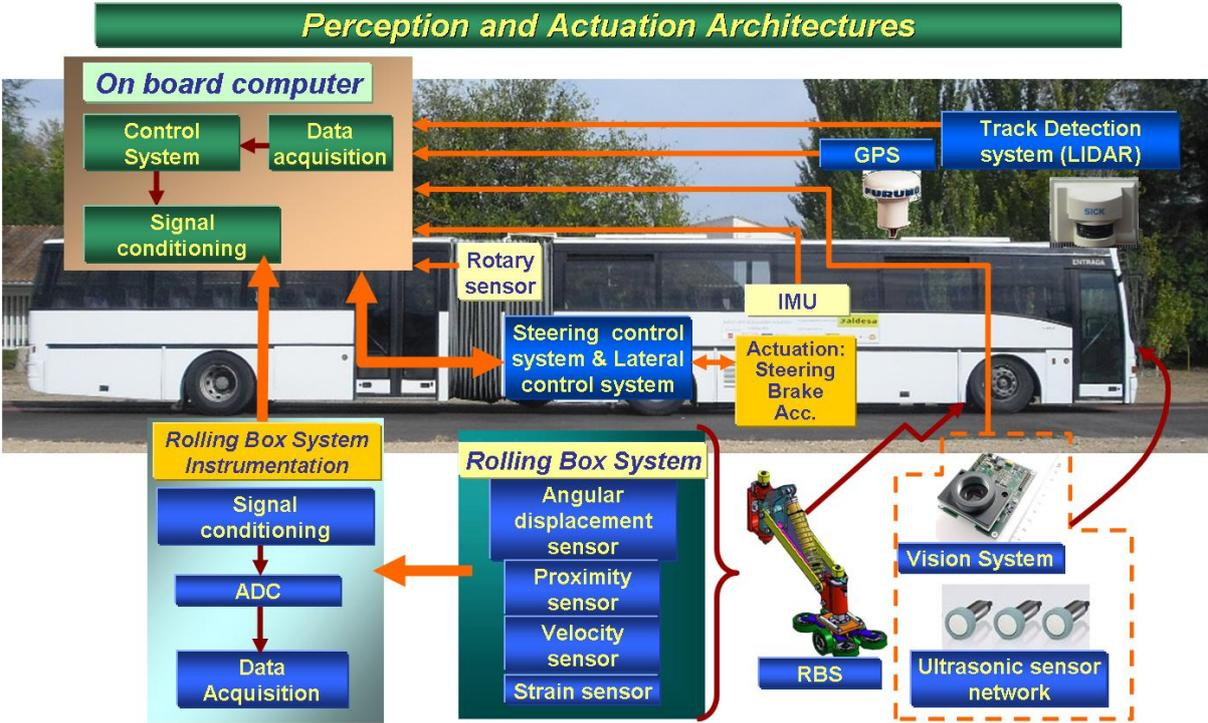
Figure 1. Architecture of the systems of perception and actuation for automation of articulated bus.
