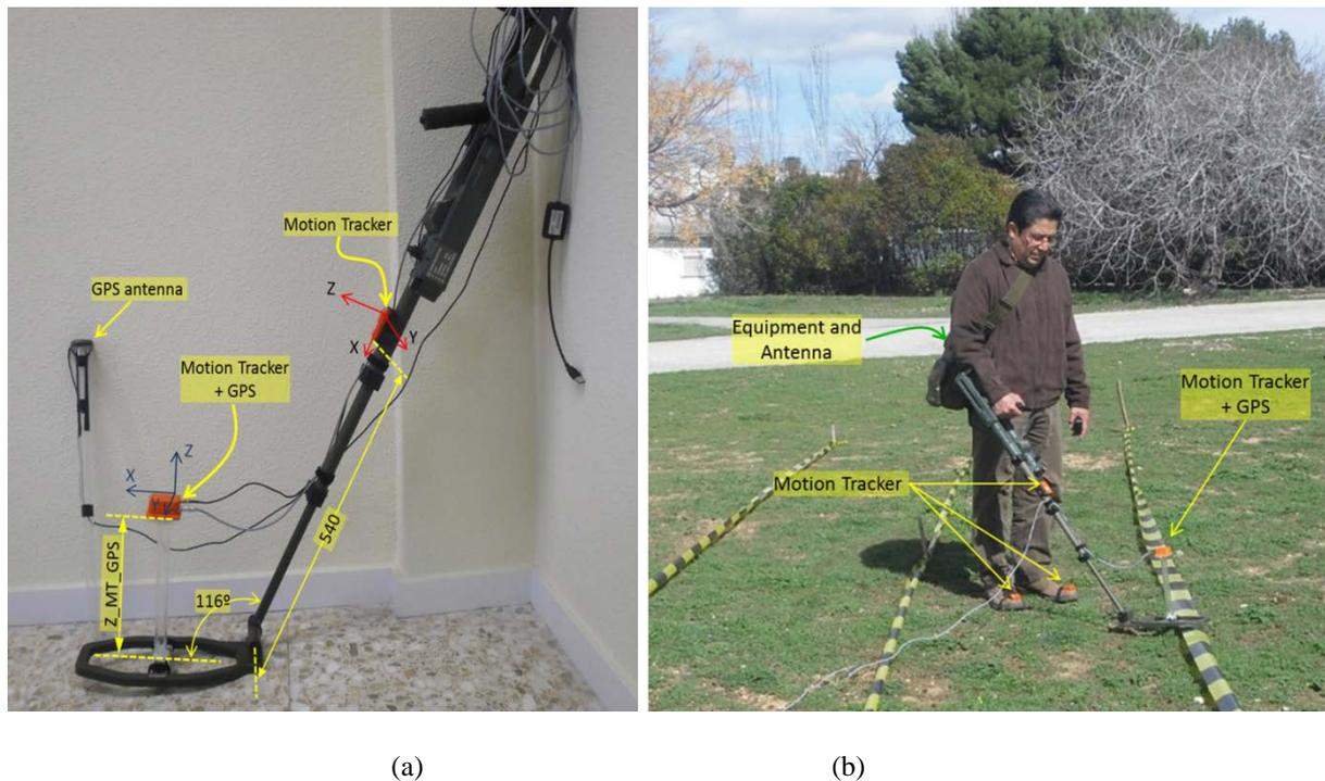
Fig. 1. (a) Hand-held detector instrumentation. (b) Operator with hand-held detector training tool during outdoor experiments at the Centre for Automation and Robotics – CAR (CSIC-UPM).
