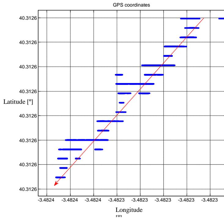
Fig. 3. GPS coordinates: Longitude and Latitude in decimal degrees. Arrow indicates motion direction.
