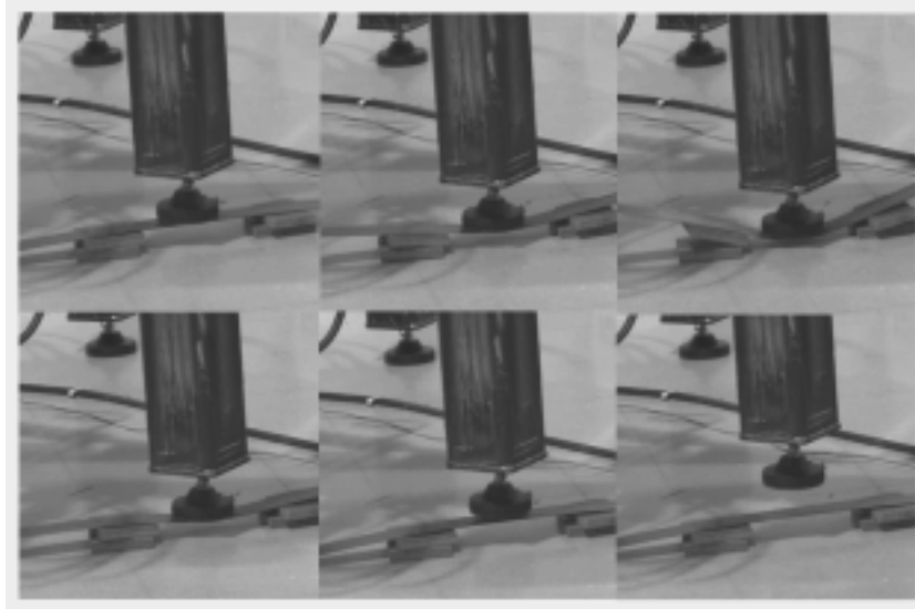
Fig. 16. Sequence showing the interaction of the leg with a flexible steel plate.
