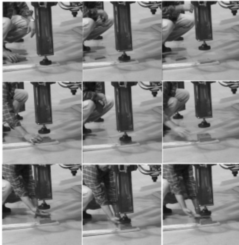
Fig. 14. Graphic sequence showing force-controlled detection of ground at different levels.
