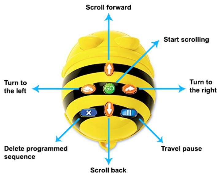
**Figure 5.** Bee-Bot® Robot: description of buttons and their functions. Source: Own elaboration.
