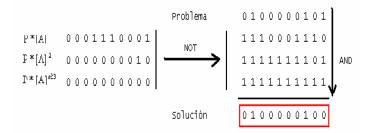
Note that for the used problem vector the most significant alarms are 2 and 8, as seen in the following graph (Fig. 10).
