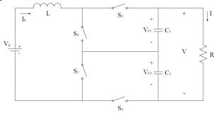
Figure 1: Two-level boost converter
