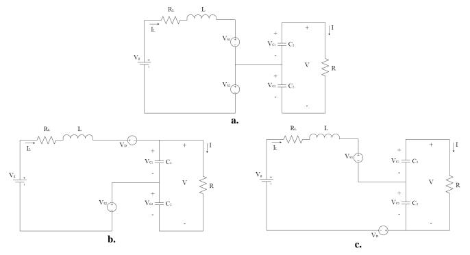
Figure 4: Loss model for each operation state of the two-level boost converter: a. inductor charging, b. capacitor 1 charging and c. capacitor 2 charging
