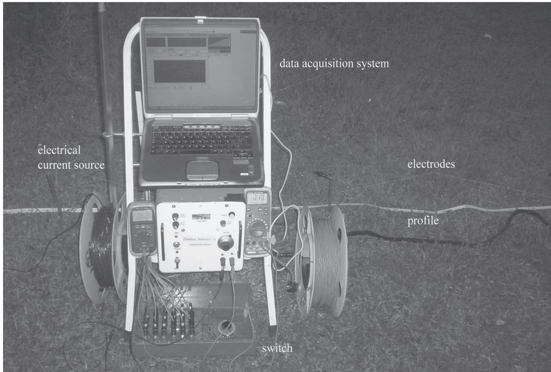
Fig. 3: Multi-electrode system used for 2- dimensional resistivity survey.
