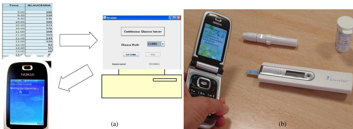
Figure 6. (a). Continuous glucose sensor simulation, (b). Communication between mobile phone and glucometer
