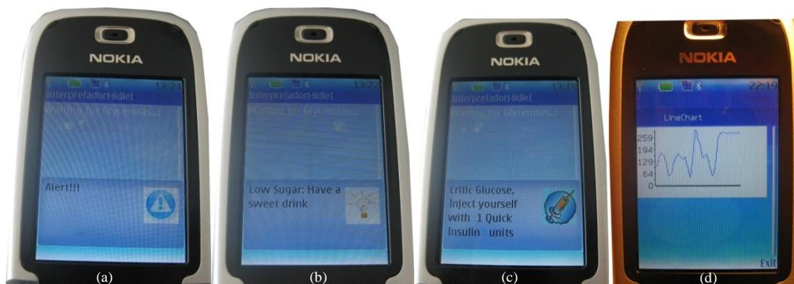
Figure 5. (a) Carbohydrate suggestion, (b). Alert module triggered, (c). Insulin dose proposal, (d). Unattended 24 hours' glucose graph
