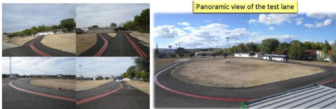
Figure 4. Partial and panoramic views of the new monorail test lane of 385 m long.
