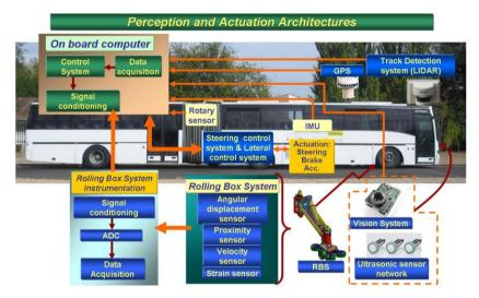
Figure 1. Proposed architecture for perception, actuation and control for the automation of articulated bus.
