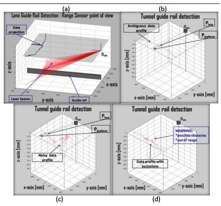
Figure 5. (a) Local *laser\_rail* world frame and its variables; (b) Ambiguous profile; (c) Noisy profile and (d) Data occlusion profile.
