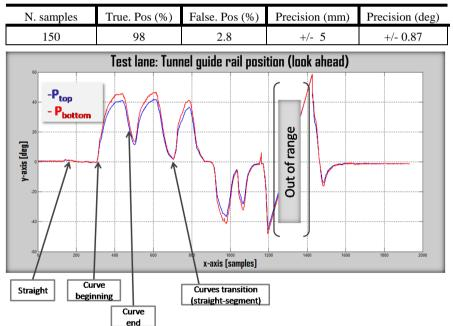
Figure 6. Tunnel guide rail detection, angles at  $P_{top}$  and  $P_{bottom}$  over the entire trajectory (see Figure 3(a)).
