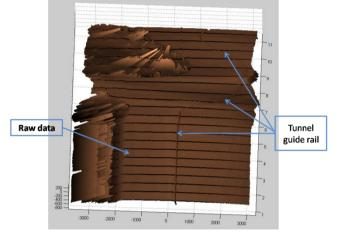
Figure 4. A 3D terrain representation from raw acquired data (top-view).
