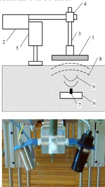
Fig. 3. Position of the metal detector on the robot. 1: metal detector, 2: robot platform, 3: support, 4: height adjusting unit, 5: pedipulator, 6: mine, 7: metal part of the mine, 8: transmit field, 9: receive field (top) and infrared sensor (down). ISR [30].
