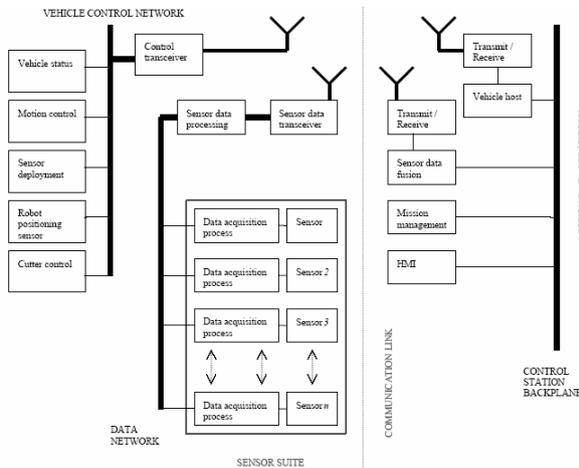
Fig. 1. Modular description of a Robotic System for the Detection of Explosive Devices
